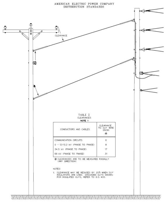
CLEARANCES BETWEEN SPAN GUYS AND LINE CONDUCTORS TRANSVERSE TO EACH OTHER ATTACHED TO SAME STRUCTURES ALL VOLTAGES
