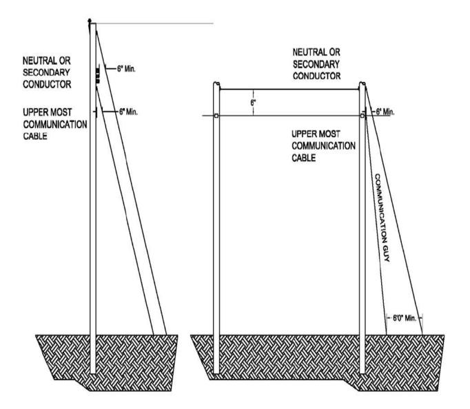
1. 6" MIN. REQUIRED IN ANY DIRECTION FROM THE HIGHEST COMMUNICATION LINE TO POWER GUYS
